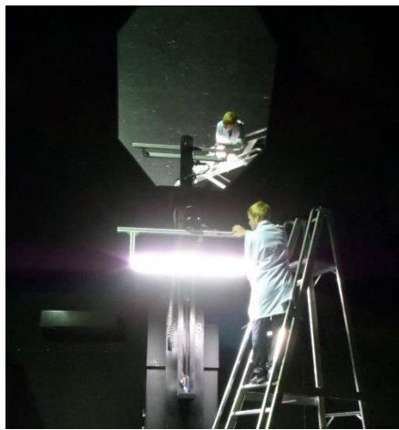
A linear downlight from Vierlight on Lux-TSI's goniophotometer
